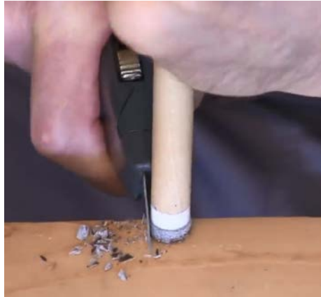
Image 5 Trimming the tip
