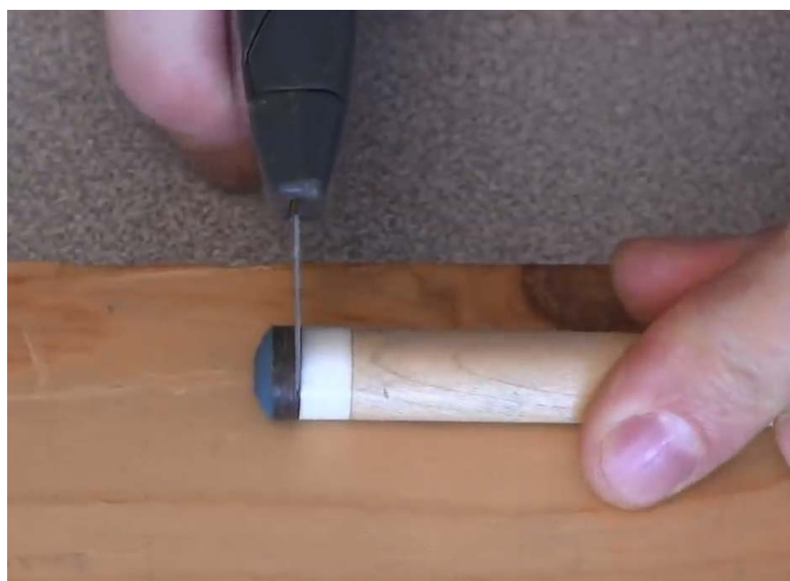
Image 3 Removing the old tip
