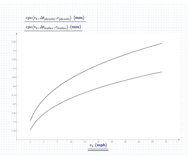
As expected, the contact patch size increases with CB speed, and is larger for a leather tip as compared to a phenolic tip. With a powerful break (25 mph), the contact patch sizes for phenolic and leather tips are approximated to be:
