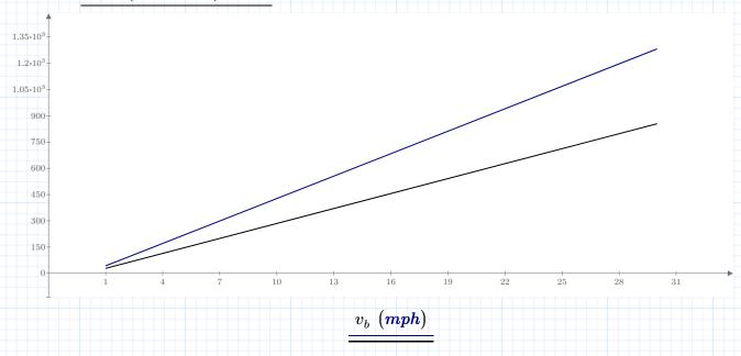
As expected, the peak contact force increases with CB speed, and is greater for a phenolic tip as compared to a leather tip. With a powerful break (25 mph), the peak forces on both phenolic and leather tips are:
