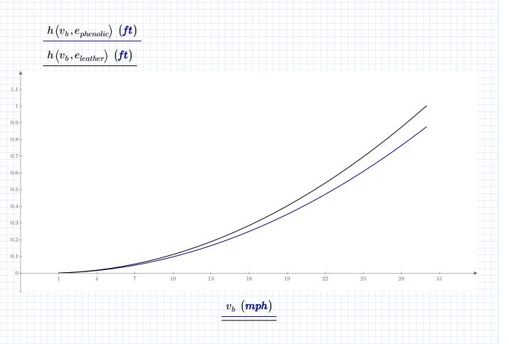
As expected, a larger drop height is required to simulate faster CB speeds, and the drop height for a leather tip needs to be a little higher compared to a phenolic tip. With a powerful break (25 mph), the required drop heights for both phenolic and leather tips are approximately:
