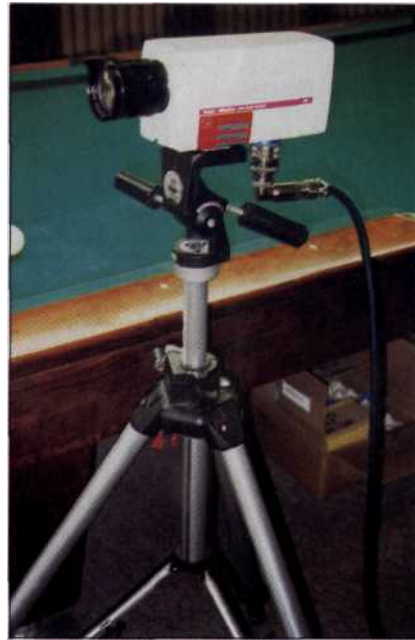
Top and below: The Kodak model 1012 Ektapro High Gain Imager with Hi-Spec processor, capable of capturing up to 12,000 frames per second.
