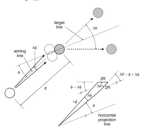
ball radius:  $R_{\hspace{-0.1cm}\tiny M}:=1.125$   $\phi$ : cut angle  $\theta$ : object ball leaving angle
