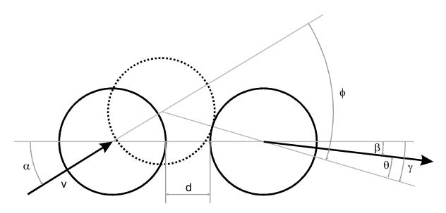
The first OB is hit with speed v at angle  $\alpha$  (relative to the original line of centers of the OBs) resulting in cut angle  $\phi$ , and impact line-of-centers angle  $\gamma$ . Cut-induced throw (CIT)  $\theta$  results in the second OB heading at angle  $\beta$  relative to the original line of centers.
