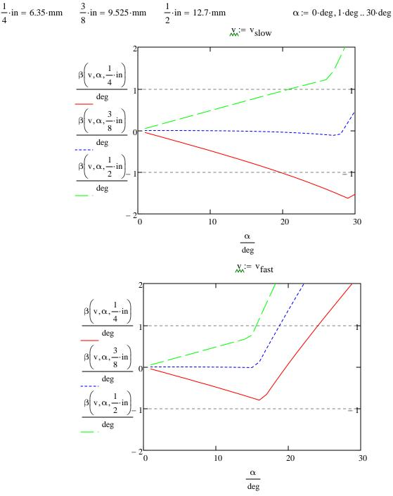
For a slow shot (top plot), a 3/8" gap results in excellent accuracy over a wide range of angles, as proven above and as demonstrated in the following video:
