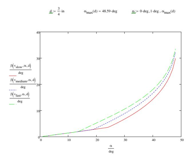
So when the gap between the OBs is larger than 3/8 of an inch (here, 3/4 of an inch), the 2nd OB always heads in the cut direction, regardless of shot speed; although, throw reduces the cut more at slower speed (except at small angles where the speed has no effect).
