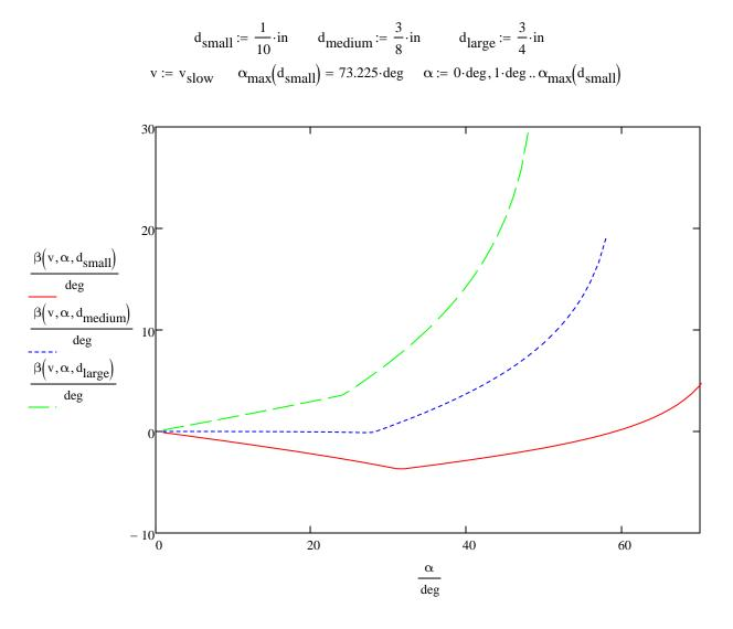
Again, only when the gap between the OBs is 3/8" (9.5 mm) does the 2nd ball head very straight (i.e., the throw and cut effect cancel) over a fairly wide range of 1st-ball angles. With a smaller gap, the throw effect is stronger at small angles and the cut effect is stronger at large angles; and with a larger gap, the cut effect is stronger at all angles.
