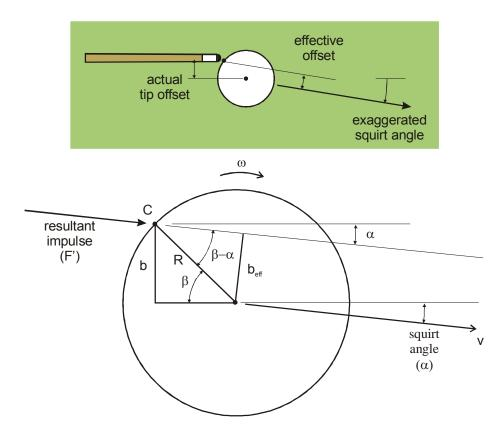
From the diagram above, the effective offset, for a cue with a squirt angle " $\alpha$ " and actual tip offset "b," is given by:
